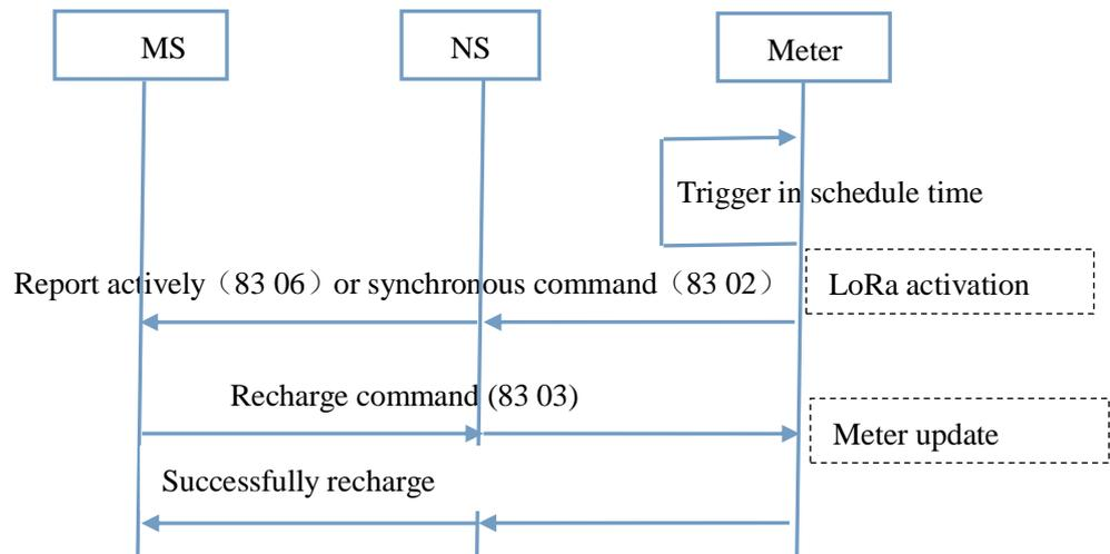
Remark: Recharge key information use DES encryption, fill the user number at the first time to recharge and complete the binding between user and meter; Check the user no. and times of gas purchasing in the follow-up recharge process, only if the times of gas purchasing in the recharge information is more than 1 time comparing with the times in the gas meter, the system judge the recharge information is valid.
